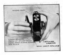
5. Next put on the back cover, sliding the cover along endwise and seeing to it that rubber pressure pad on cover presses down on lip of cartridge. Insert hook in case and pressing down on catch lock cover securely.
